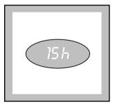
The delay time is displayed for 3 seconds, then the duration of the selected programme reappears. After you have pressed the START/PAUSE button, the
